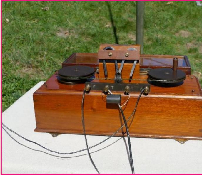
**Photo N° 9 the magnetic detector in operation**
