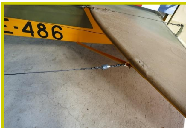
Insulator connected to the tail boom
