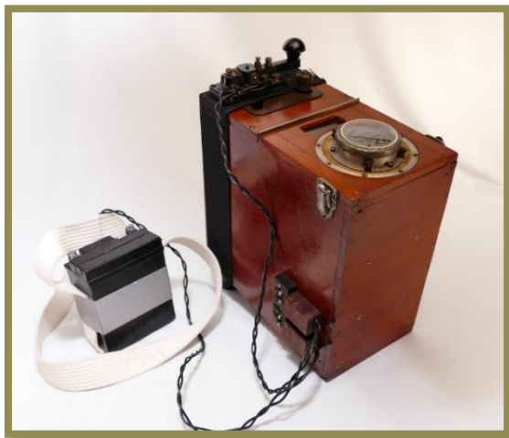
The Marconcina with 12 Volt battery and telegraph key
