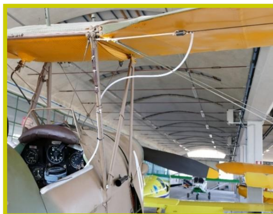
Interplane strut to allow the antenna cable to enter the observer's cockpit
