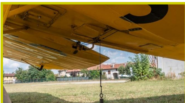
The 25-metre antenna, with a weight of about 300 g, which comes out of the biplane's cockpit
