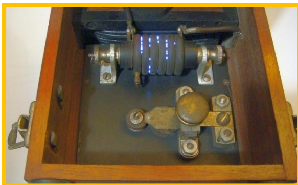
6 disc discharger all connected between 4, or 5, or 6 discs.
